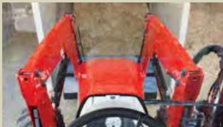
The main loader arms are constructed of two U shaped, high strength alloy steel channels fitted together and welded on the inside for a wide profile with a clean, strong appearance.
