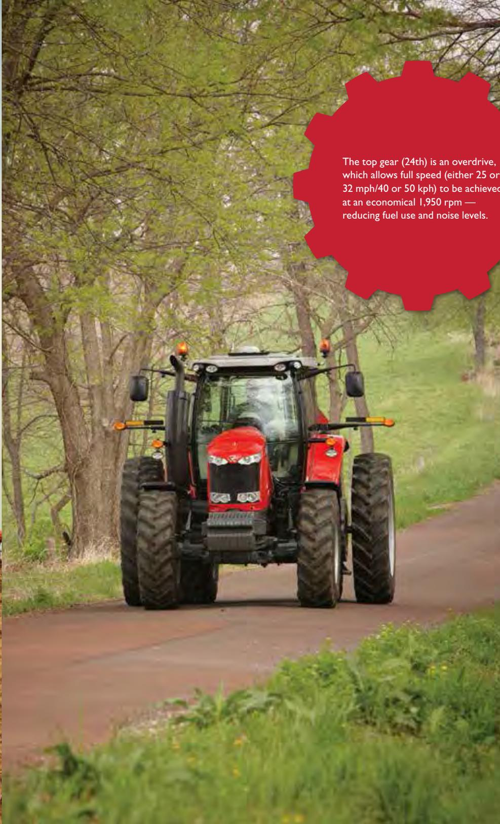
The top gear (24th) is an overdrive, which allows full speed (either 25 or 32 mph/40 or 50 kph) to be achieved at an economical 1,950 rpm — reducing fuel use and noise levels.
