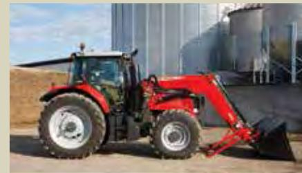
Loader mounting is fast and easy, thanks to our unique "Lock and Go" connection system and a quick connection option, which groups all hydraulic couplers into a single block coupling.
