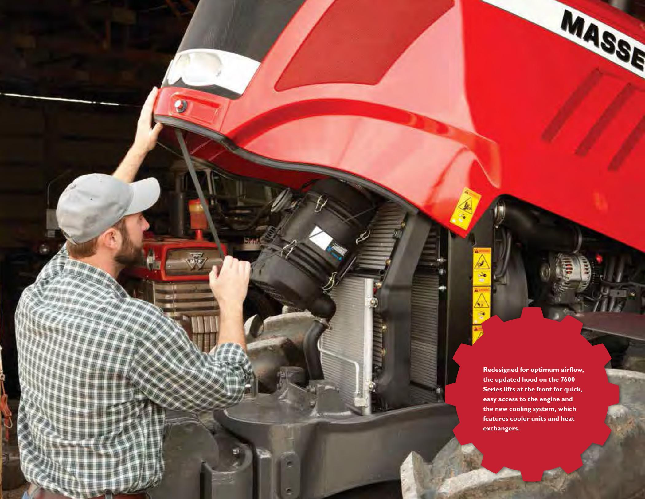
Redesigned for optimum airflow, the updated hood on the 7600 Series lifts at the front for quick, easy access to the engine and the new cooling system, which features cooler units and heat exchangers.
