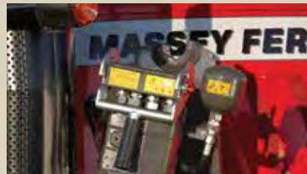
A centrally located valve unit protected by the cross tube and hidden under a cover connects all functions at one point for easier service and synchronized flow between the left and right sides, regardless of the load, oil temperature or hydraulic pressure.
