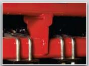
**Heavy Frames** The 7" x 7" x 3/8" main frame and 3" x 5" x 3/8" opener frame tubes are bridged for extraordinary strength.
