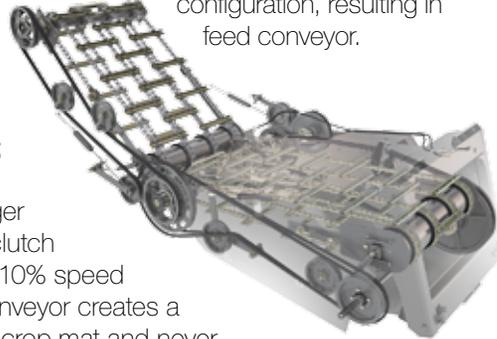
The rear feed conveyor drive can take 50% more horsepower; the 2B belt drive features five new pulleys, two belts and a larger Walterscheid feeder house slip clutch delivering 25% more torque; the 10% speed differential from the front feed conveyor creates a hyper-pull system, keeping a flat crop mat and never changing direction but feeding the Tritura™ processor quicker and reducing pinch points for greater capacity.
