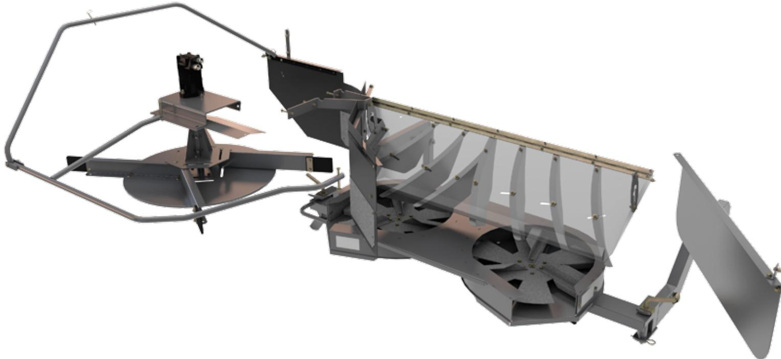
The S8 Super Series features a completely redesigned 2-speed chopper for greater residue chopping demands when required. For high speed chopping, the smaller 7 1/2-inch chopper drum features 24 knives, a 50% increase, for greater chopping and a 16% increase in speed to 3,250 rpm to create enough vacuum pressure to pull residue on through and keep the processor cage clean, optimizing processor performance.
