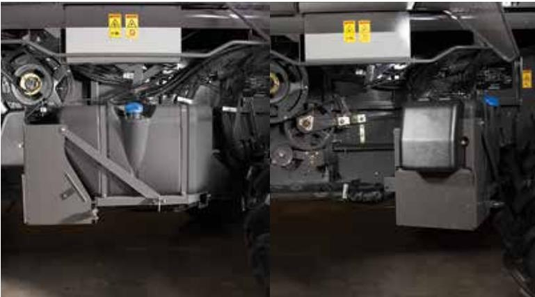
Gleaner S8 models feature a new integrated tool box located in the front of DEF tank for easy ground level access. The DEF tank support includes a pivoting feature that swings out and away from the machine for easy access to all the lower drives and drains for clean grain and tailings elevator troughs for improved serviceability.
