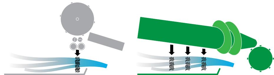
The same issue of where grain drops from the rotor affects the effectiveness of the shoe. The Gleaner always drops its grain and material in the same position. Axial combines tend to unevenly distribute grain to the cleaning shoe. This can cause grain loss out the back of the combine.
