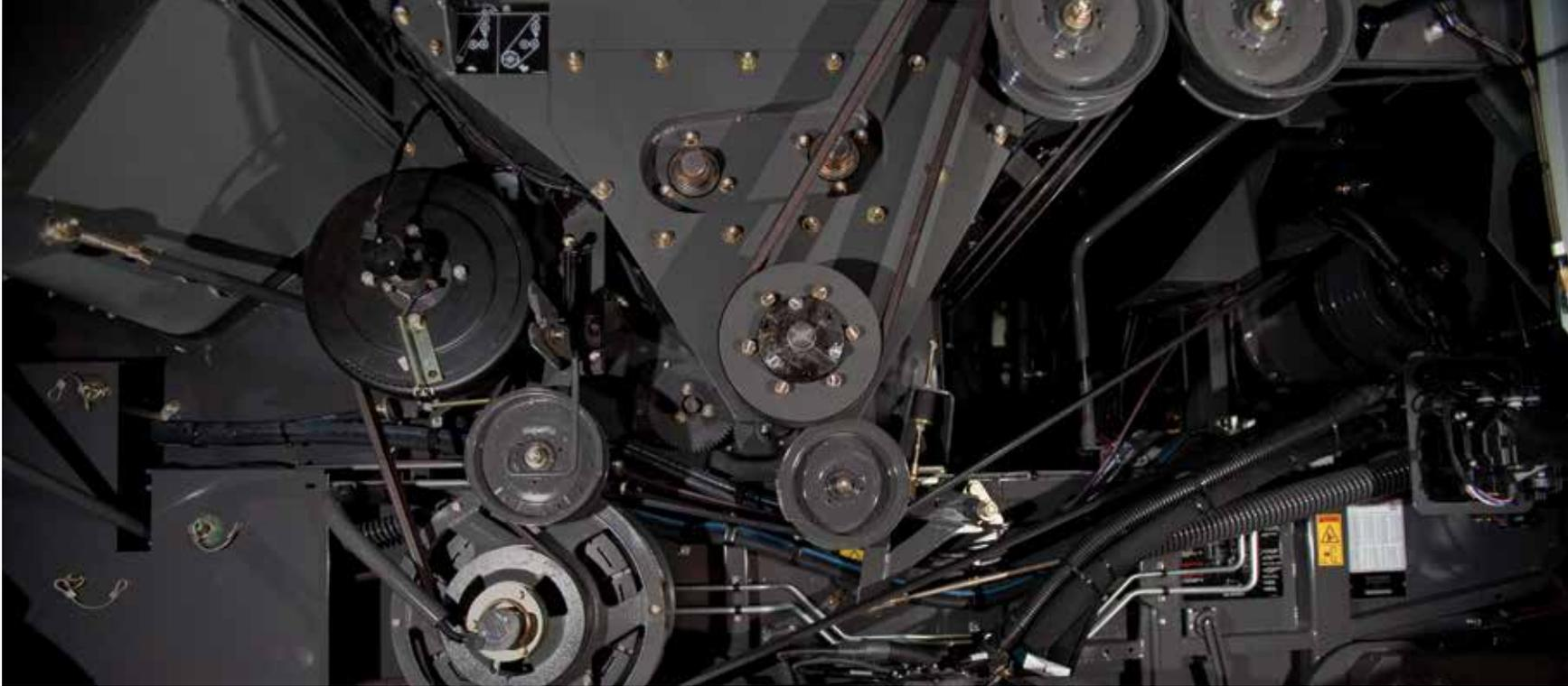
Because Gleaner Super Series combines use straight-through shafts, changing belts and making adjustments to the machine is easier, which can be done with both feet on the ground, taking less time away from your harvest. The S8 Super Series rotor can be removed in literally a fraction of the time it takes to remove a rotor from our competitors' combines.
