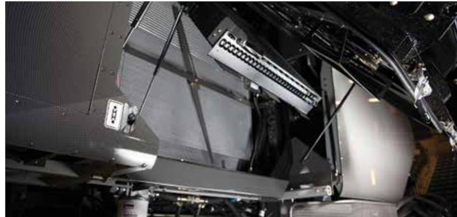
The entire rotary screen box and coolers pivot out for easy service inspection. Exclusive SmartCooling™ eliminates the need for daily cleaning of the radiator, coolers and rotary screen even in heaviest soybean dust and chaff.
