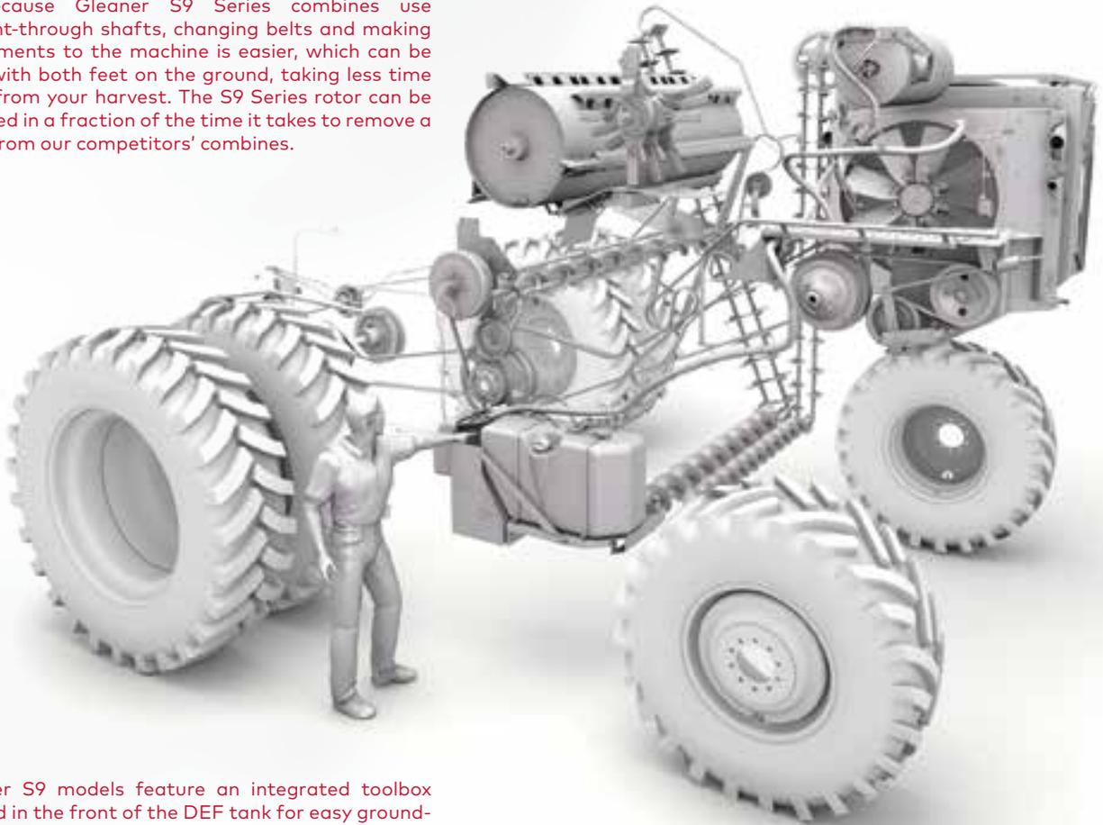
Gleaner S9 models feature an integrated toolbox located in the front of the DEF tank for easy ground-level access. The DEF tank support includes a pivoting feature that swings out and away from the machine for easy access to all the lower drives and drains for elevator troughs.
