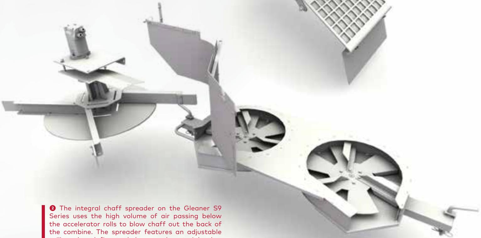
2 The integral chaff spreader on the Gleaner S9 Series uses the high volume of air passing below the accelerator rolls to blow chaff out the back of the combine. The spreader features an adjustable tailboard and fins to help spread material other than grain (MOG) into a wider swath as it leaves the machine. There is no stripping of material and no mechanical drives that rob horsepower as in competitors' designs.
