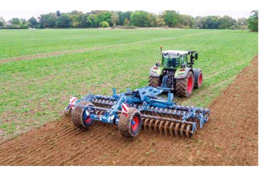
The Heliodor compact disc harrow from LEMKEN uses two rows of discs individually mounted to leaf springs. This system provides a uniform cultivation depth, whilst allowing individual discs to ride over stones when necessary. During stubble cultivation the discs ensure soil and vegetation are evenly and intensively mixed.
