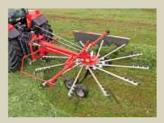
Designed for smaller tractors without hydraulic valves, our new RK3802 single rotor rake provides an economical upgrade from vertical fold wheel rakes. You'll appreciate its three-point hitch lifting, requiring no SAV or DAV.
