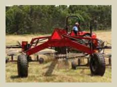
All our dual rotor models are equipped with a transport chassis with steerable rear wheels. This feature gives you greater maneuverability on tight turns while raking, or during transport from field to field.
