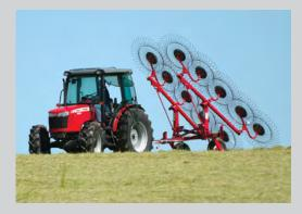
**ONE SINGLE-ACTING CYLINDER** folds both wings for easy transport (available on 1508, 1510 and 1512 models).
