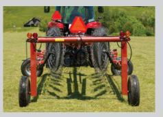
**FOLDED FOR TRANSPORT,** the 3986 and 3983 models fold to 8 feet — all without ever leaving the tractor seat.
