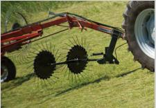
AN OPTIONAL CENTER KICKER WHEEL is available on both 3900 Series wheel rakes, as well as all 1500 Series rakes to turn the entire windrow and eliminate any wet spots beneath unraked crop.
