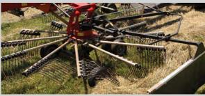
**LONG TINES** feature smooth front surfaces for long life and smooth crop release, creating a clean, uniform windrow. Our tine design also allows easy individual replacement of the tines, making it easier to maintain.
