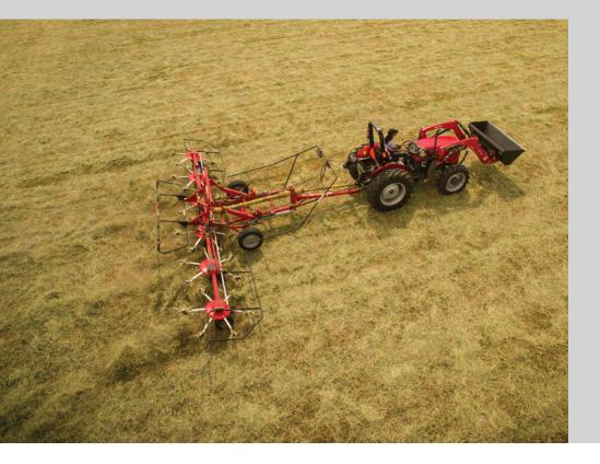
All models are simple to set-up and adjust for quick and efficient ground coverage. Four, six, eight and 10-rotor models also feature synchronized lifting of exterior rotors via a centralized hydraulic lift system and pressure cylinders to ensure optimum performance and eliminate one-sided loads — even on slopes.
