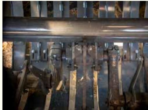
**Enhanced throughput** with a 14% faster packer crank, feeding crop into the pre-compression chamber.
