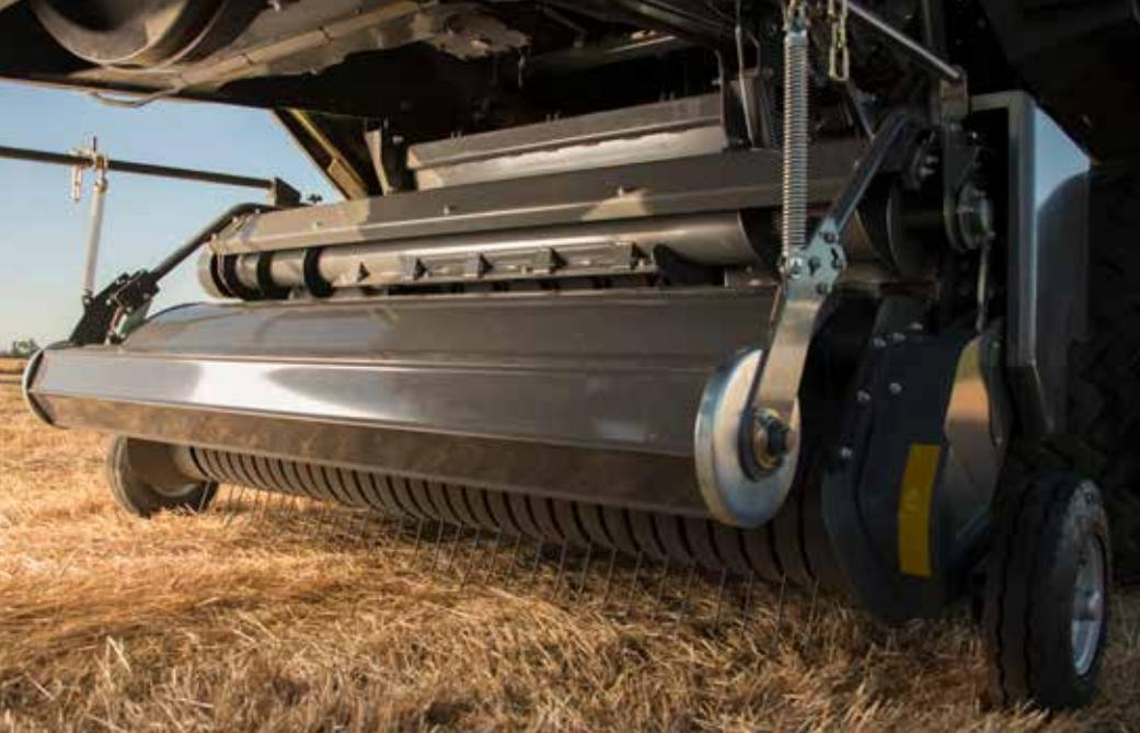
The new OptiFlow™ Pick-up has 25% more pick-up tines than our XD baler, to improve crop gathering performance at high speeds. Add to that a full-width powered top auger that enhances throughput in large windrows — and a new wind guard with large-diameter roller for consistent crop flow. It all works together to deliver greater capacity.
