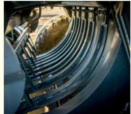
**New pre-compression chamber** features thicker stuffer chamber wrappers with support ribs for increased durability in tough crop conditions.
