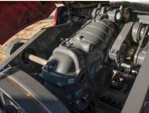
**Ultra™ Gearbox** with our industry-exclusive torque-split gearbox design provides a new way of reliably transferring massive amounts of power through a package intended to operate without excess size and weight.
