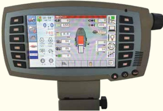
Working with all ISO-compliant tractor monitors, the easy-to-use 2370 Ultra HD software displays everything needed to control bale quality: steering arrows, flakes per bale, total bale count, density pressure, plunger position, previous flake size and current bale length. Better control equals better bales and quicker turnaround times.
