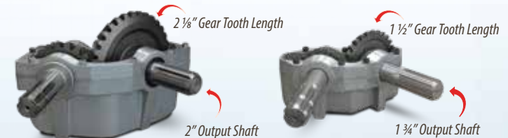
J&M Heavy-Duty Gearbox 362 HP Static/168 HP Dynamic
