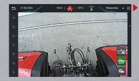
**Video mode** — Pictures from the on-board camera can be displayed on the console screen, allowing operators to monitor complex implements or simply improve efficiency when reversing.
