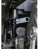
**CAB SUSPENSION** brings extra comfort. Two types available: mechanical and active mechanical.
