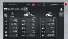
Memorize data and settings — An unlimited number of user setting configurations enable the system to record information during operation on area worked, fuel use, hours worked and much more. All the settings and parameters can be stored by the Datatronic 5 terminal and recalled to find a previous setting.
